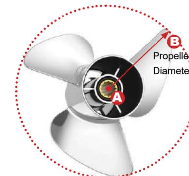
(Line A-B x 2 = Propeller Diameter)
