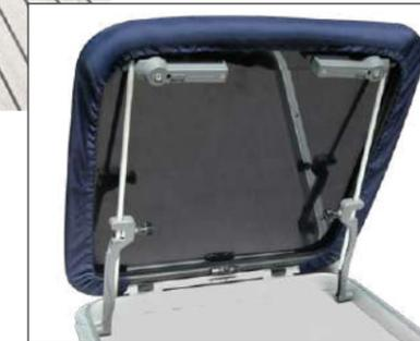
Oceansouth's unique design allows the hatch cover to stay in place when the hatch is opened and remain firmly secured around the hatch when closed.
